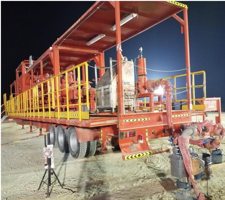
**Separator with associated Gas Orifice Meter &
